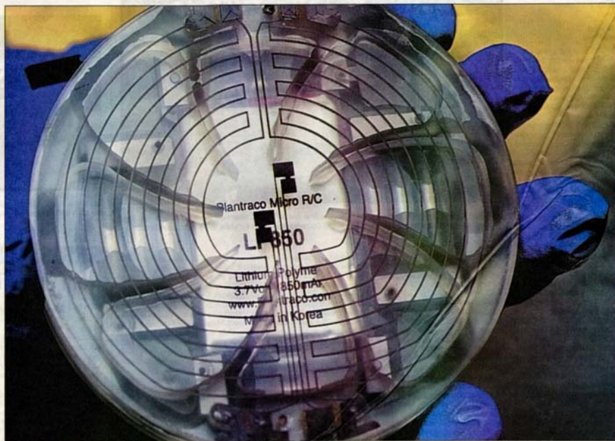
This prototype of a satellite propulsion module built by The Aerospace Corp. uses glass and ceramic components to make a significantly lighter and smaller satellite.
