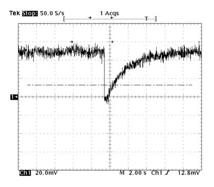
A photodiode monitors the MOT fluorescence as the trap loads
