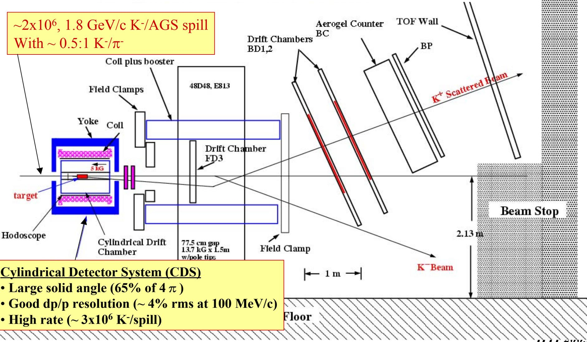
**Cylindrical Detector System (CDS)**
