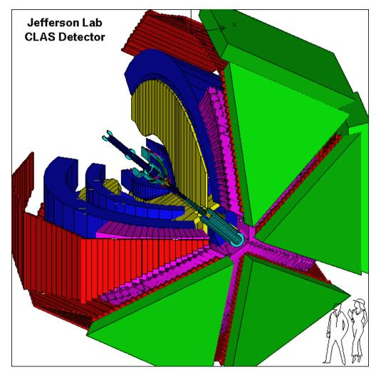
Toroidal magnetic field (yellow coils) bends charged particles toward or away from beamline
