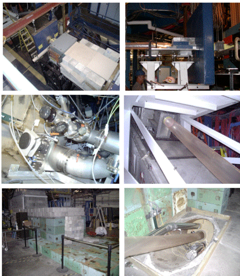
Figure 42: Photographs taken during engineering work, Top-left: from right to left are second chicane tunnel, second Italian dipole, rad-phi collimator, rad-phi wall and helium bag. Top-right: cleanup collimator downstream of rad-phi wall, Mid-left: tagger flanges and vacuum pipe, Mid-right: tagger vacuum box window and helium bag, Bottom-left: tagger bunker shield, Bottom-right: tagger dump can. Photos are provided by [45].
