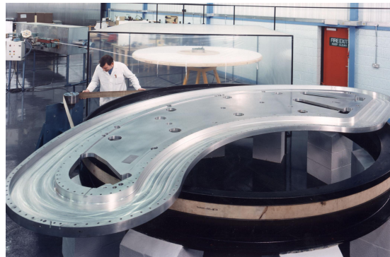
Figure 2-5: Construction of the coils of the Torus magnet
