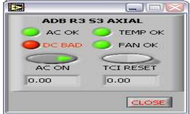
Figure 5: Individual-Crate-Front-Panel with an error
