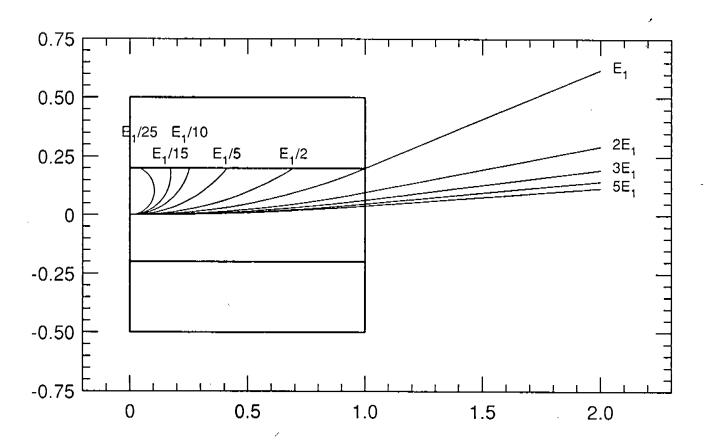
Figure 4. Typical electron trajectories in the pair spectrometer magnet whose geometry is described in Section 3.3. Each trajectory is labeled with its energy in units of the "corner" energy  $E_1$  ( $E_1$  = 780 MeV for B = 1.0 T).
