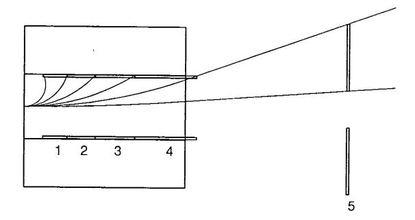
Figure 5. Positions of counters with approximately equal counting rates. The trajectories shown define the boundaries between the energy bins (see Table 2). (a) 5 equal-rate bins from E = .0513  $E_0$  to 5.13  $E_0$  (40 MeV to 4 GeV at B = 1.0 T). (b) 10 equal-rate bins between the same limits.
