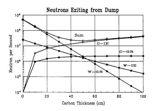
Figure 1. Neutrons exciting the tagger beam dump as a function of the thickness of the carbon absorber. The neutrons come either from the tungsten (W) or carbon (C), and are created either by the giant resonance reaction (GR) or intermediate energy pion production (IE).
