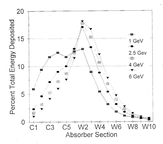
Figure 2. The percent of total beam energy deposited in the beam-dump absorber plates for several different incident beam energies. "C" indicates on of the 5 carbon absorbers, "W" indicates the associated tungsten absorber.
