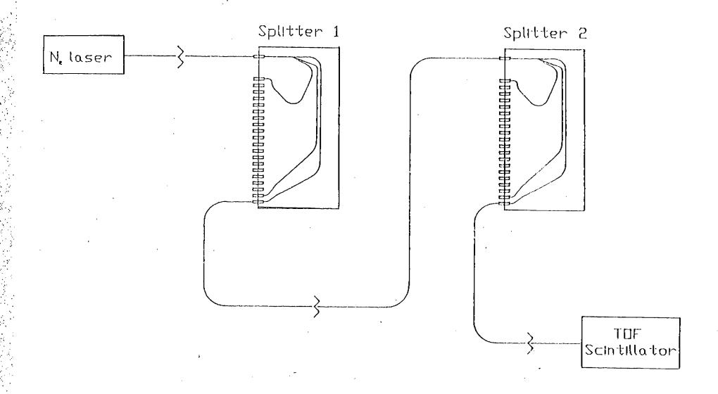
Figure 1. Schematic of Test System
