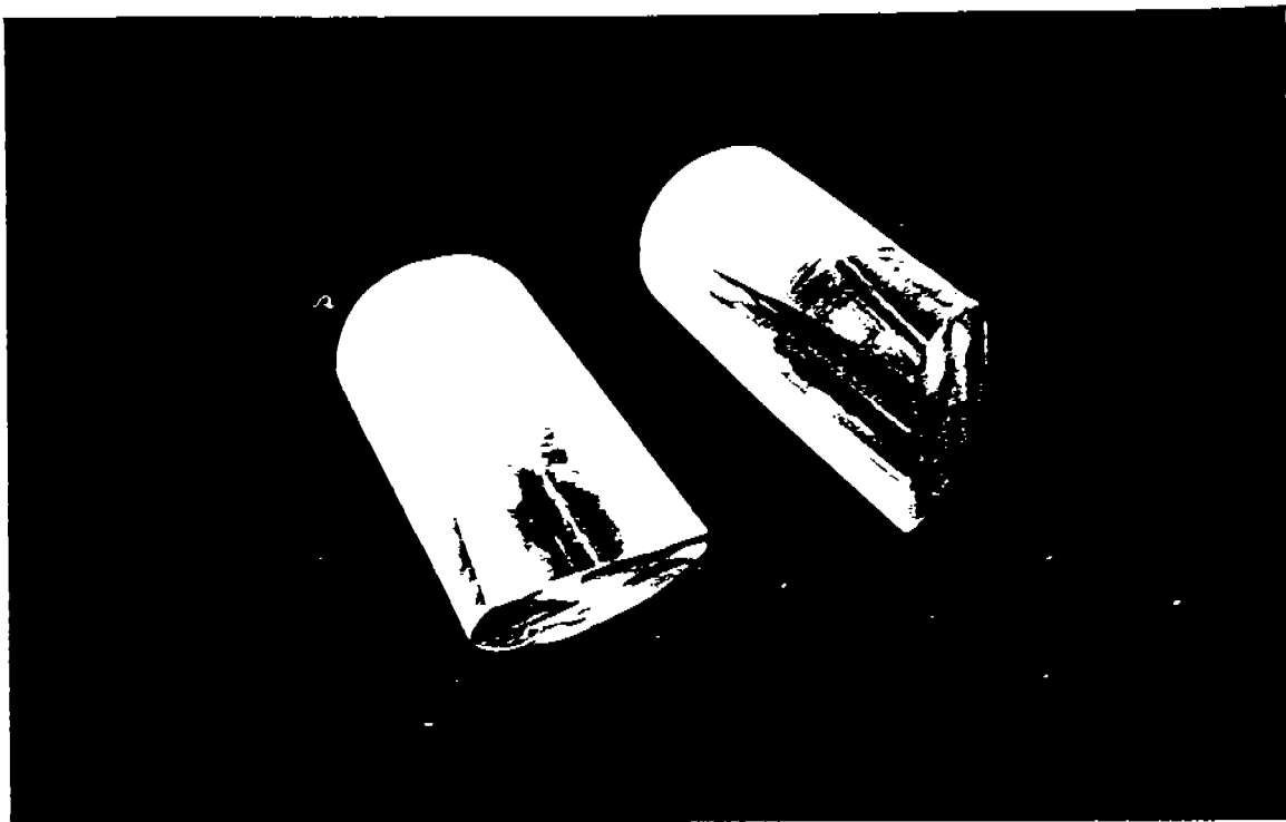
Figure 7. Short, cylindrical guides with 30^\circ angles. These were at one time seen as the most simple solution for the LATOF scintillators. Light losses due to mismatch between scintillator (5 x 20 cm) and cylinder (3" diameter) cross sections.
