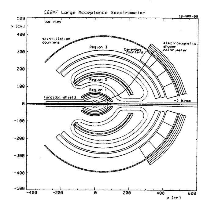
Figure 3: Midplane slice of the CLAS detector as viewed from the top. The dotted lines show the projection of the coil contours on the midplane. The trajectory of a 1 GeV/c particle is shown in a nonzero magnetic field. [This figure is from Fig. E2 of the Hall B Conceptual Design Report, April 1990].
