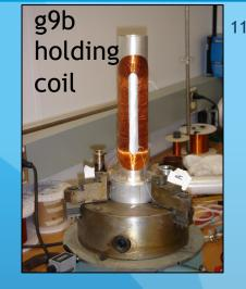
Butanol dripped into LN<sub>2</sub> bath and then cooled to <1K and LN<sub>2</sub> is replaced by LHe bath
