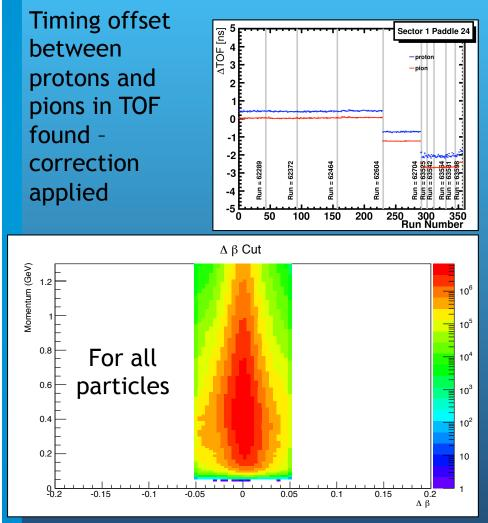
Delta Beta Cut for Kaons deltabetakaon Momentum Entries 1.685952e+07 -0.001221 Mean x Mean y 0.56 RMS x 0.02259 RMS v 0.3243 For 103 Ξ 0.8 kaons Before 10<sup>2</sup> 0.6 0.4 10 0.2 -0.06 -0.04 -0.02 0.02 0.04 0.06 0 Delta Beta  $\Delta \beta$  Cut for Kaons
