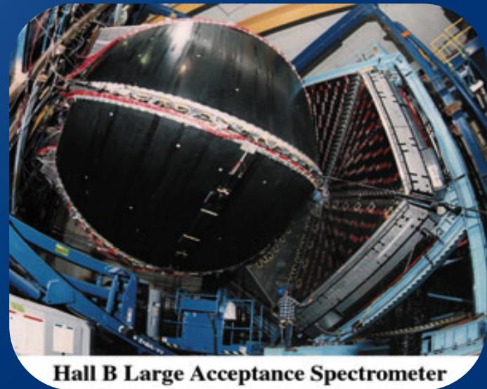
Open ( $e, e'$ ) trigger, Large-Acceptance, Low luminosity ( $\sim 10^{34} \text{ cm}^{-2} \text{ sec}^{-1}$ )
