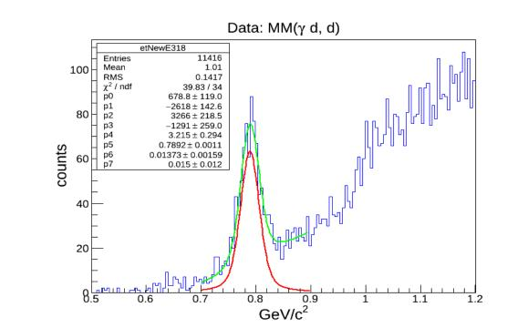
Obtaining the yield for each energy and momentum transfer (t), allows the differential cross section to be determined.
