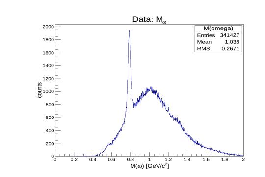
These are binned in different incident photon energy ranges and momentum transfer bins. A third order polynomial function is used to fit the background while the signal events are extracted using a Voigt profile.
