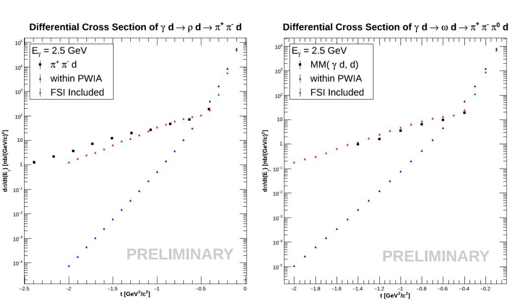
The red points are results obtained by including the final state interaction while the blue points represent results within planewave Impulse approximation [7]. The black points are the preliminary results obtained from g10 data set for  $E_{\gamma}$  centered at 2.5 GeV.
