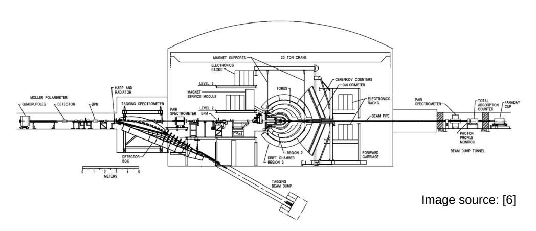
The beam is sent to bombard a liquid deuterium target. The reaction products are tracked by CLAS. Detection consists of determining a particle's TOF, momentum, and track information.
