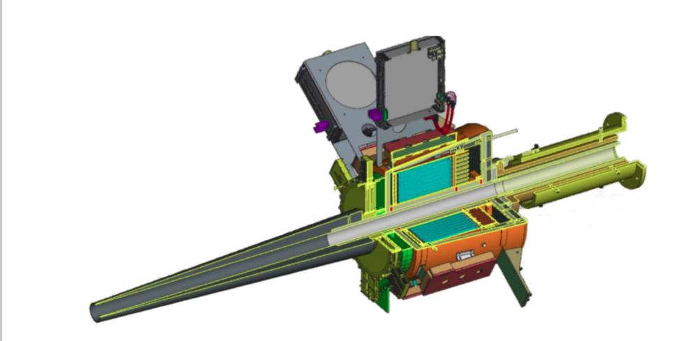
The FT has been designed to detect electrons and photons scattered at polar angles from 2° to 5° and to meet the physics goals of the hadron spectroscopy program.[2][3]
