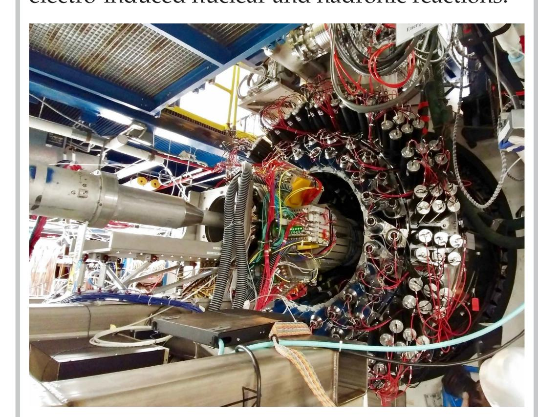
This spectrometer provides efficient detection of charged and neutral particles over a large fraction of the full solid angle (forward polar angle up to 125° with full azimuthal coverage)[2].
