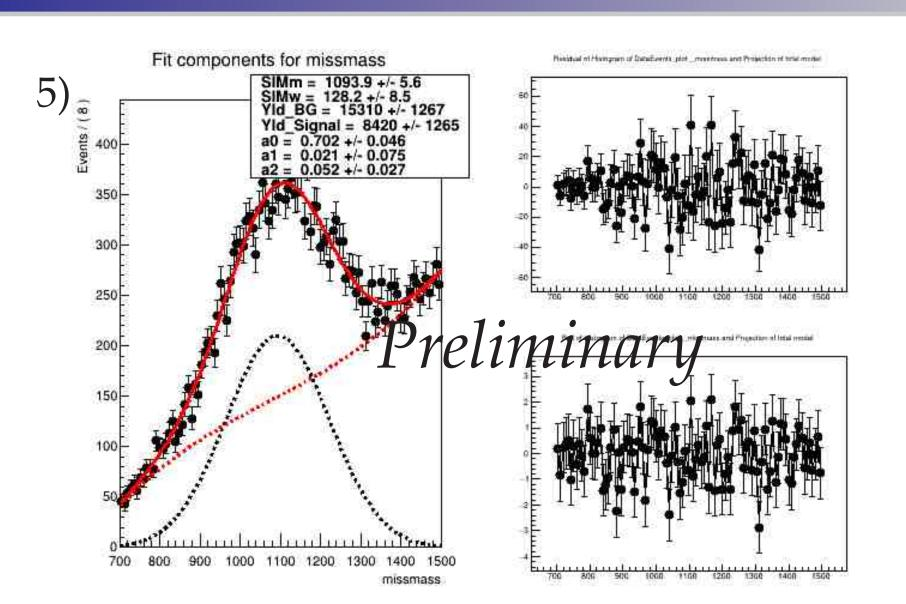
Using sPlot, a useful tool from Brufit[4], it was possible to extract clean data from the Fig. 2b. The sPlot procedure is shown in Fig. 5, where the proton peak, in black, is clearly extracted from the background, in red. Another example of the cleaning process is shown in Fig.6.
