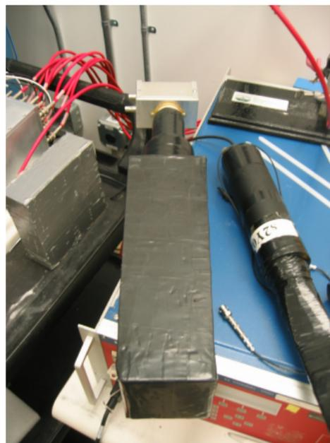
**Figure:** The CsI detector with old PMT.
