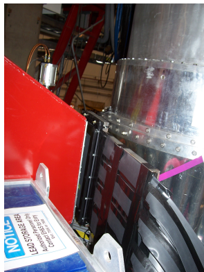
Figure: Forward tracker in position between Čerenkov snout and target OVC
