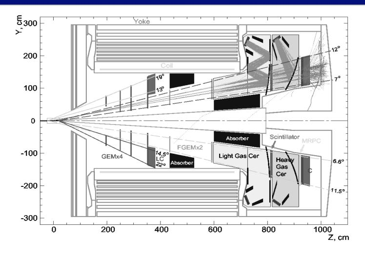
Forward angle, 7 <  $\Theta$  < 20 degree  $2\pi$  azimuthal coverage
