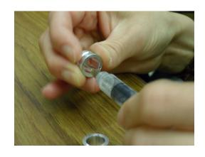
The needle should slide in and out easily. If It does, the ports are ok.
