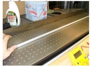
3. Push the tube lightly up against the straightedge to see if the tube is bowed. Rotate it to make sure that it is not bowed in any direction. If the tube separates from the straightedge, try to fit the 0.1" dowel in between the tube and the straightedge as this is the maximum amount of bow that can be tolerated. If it fits without pushing the tube away, reject the tube.
