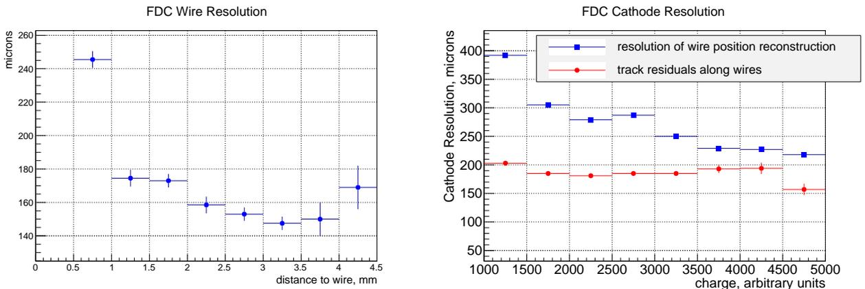
Figure 5: The FDC position resolutions: (left) from wires in  $x$  direction,  $\sigma_{wire}$ , as function of distance to the wire and (right) from cathodes,  $\sigma_{cathode}$ , in  $x$  (blue) and  $y$  (red) direction as function of the hit charge. Cathode x-resolution should be scaled down by factor of 3.86 to compare with y-resolution.
