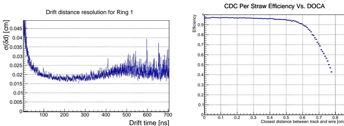
Figure 3: The position resolution,  $\sigma_{r\phi}$  of the CDC as a function of drift time.
