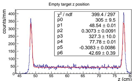
Figure 4: The  $z$  resolution at the target can be extracted from the empty target runs. The width of the thin target walls represent a measurement of  $z_{vert}$  of 3 mm.
