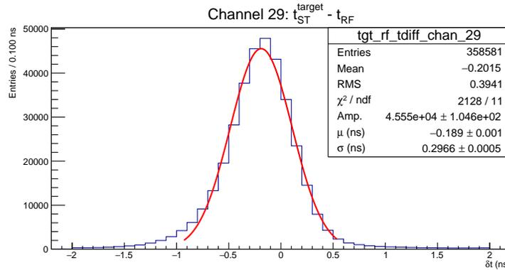
Figure 1: The time resolution of the start counter element 29 showing 300 ps resolution.
