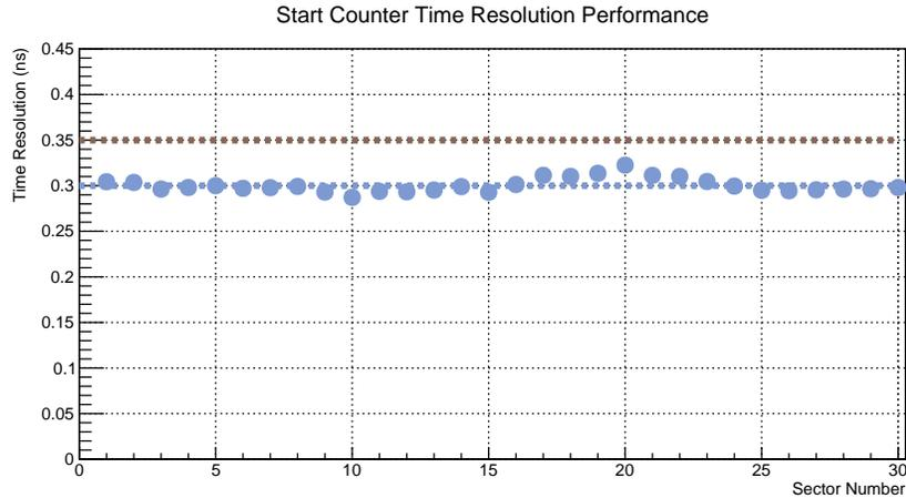
Figure 2: The time resolution of the start counter as a function of the start counter element number. The brown dashed line shows the design resolution, the blue points show the per element resolution.
