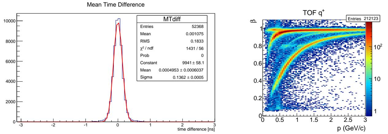
Figure 7: (left) The time difference between the summed time in the two layers of time-of-flight paddles. The  $136\text{ ps}$  sigma measurement corresponds to  $96\text{ ps}$  time resolution per layer. (right) The  $\beta$  versus  $p$  plot for positive particles. Clear bands are seen for  $e^+$ ,  $\pi^+$ ,  $K^+$  and  $p$  (top to bottom).
