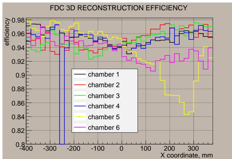
Figure 6: The combined (wire and cathode) 3D hit reconstruction efficiency for the six chambers of third FDC package vs wire position. The dips in the efficiencies correspond to bad cathode channels, most numerous in this package.
