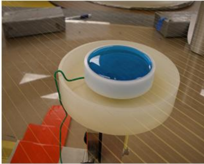
Figure 4.39: Wire deadening: a container filled with \text{CuSO}_4 is raised against the wires; voltage is applied between the sense wires and a copper electrode inside the container.
