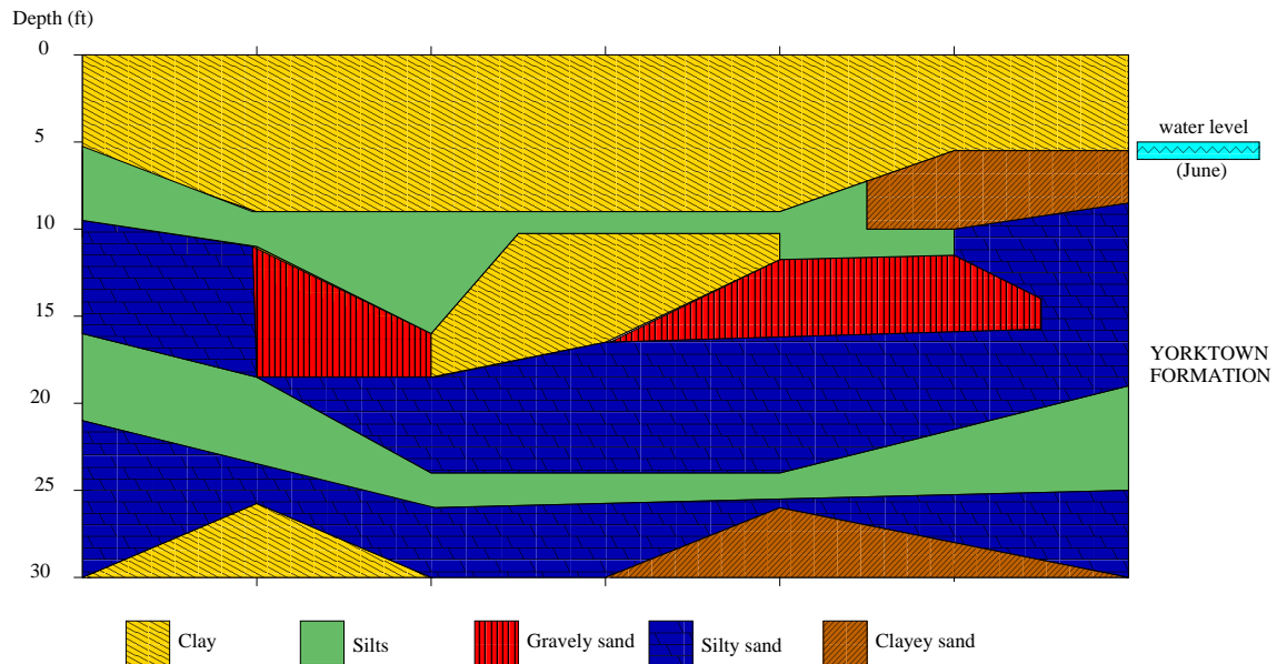
Figure A.7: Typical composition of soil under the HALL D construction site as a function of depth. Note that the horizontal dimension covers the distance from the accelerator to the building. The result of the geotechnical analysis shows that buildings at grade level will require support piles, driven approximately 15-20 m into the ground.
