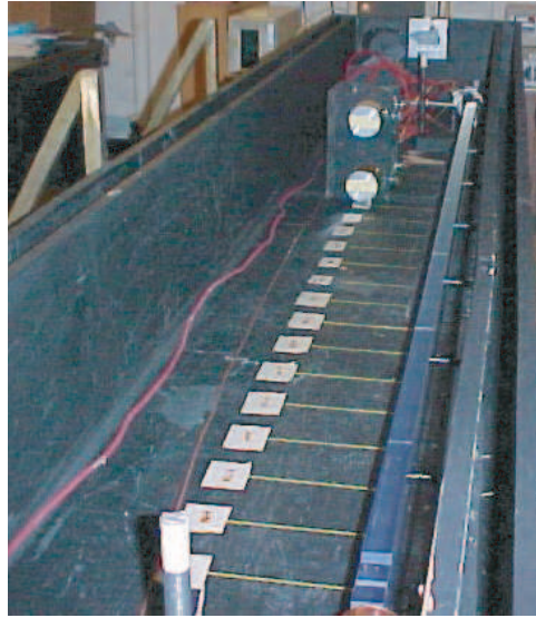
Figure 4.47: Part of the cosmic ray test facility showing a light-tight box inside of which is a 2-m long scintillator bar, read out at both ends, as well a trigger telescope with two small scintillation counters that can be positioned along the bar.
