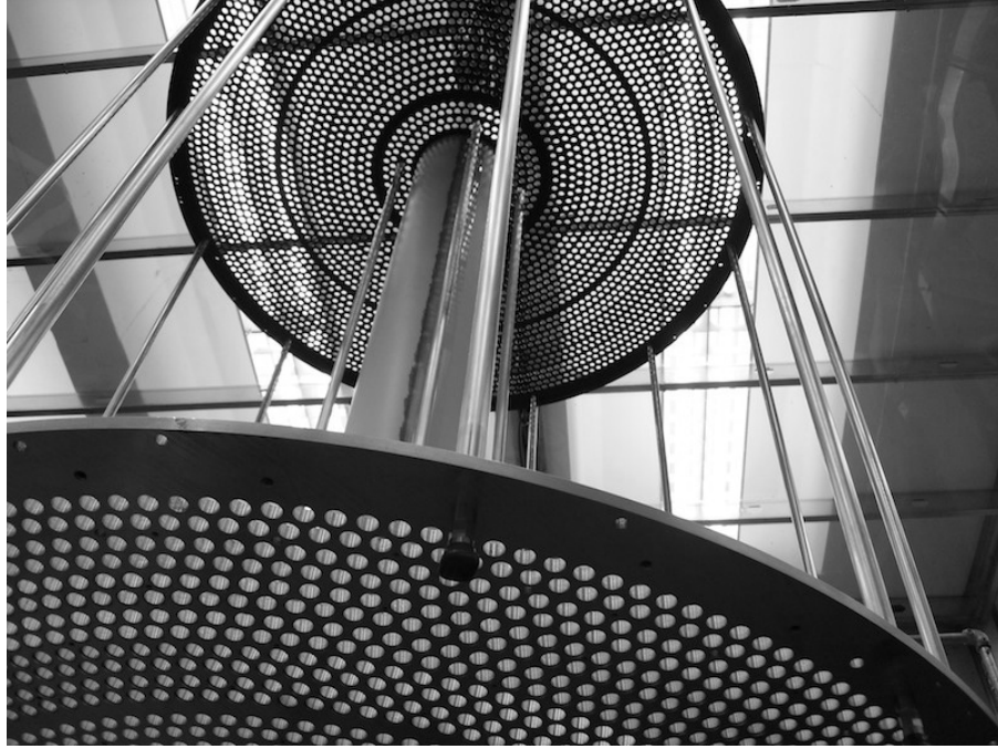
Figure 4.30: CDC frame prior to the installation of the straw tubes.
