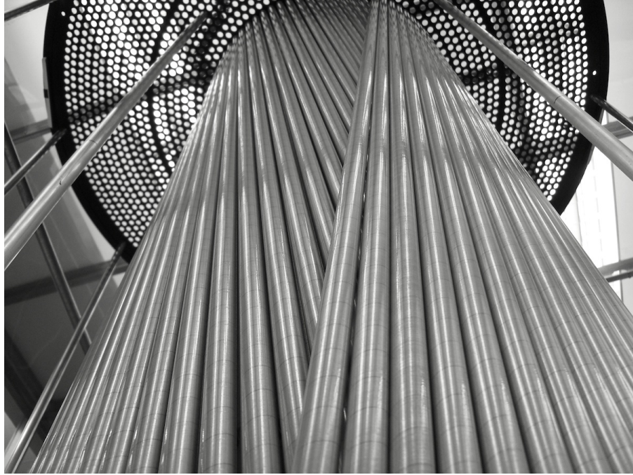
Figure 4.32: Straw tubes in stereo layers 8 and 9.
