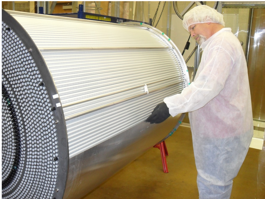
Figure 4.33: Straw tubes in axial layers 28, with one half of the outer shell in place.
