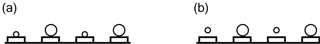
Figure 1: Two scenarios for positioning the sense and field wires relative to the solder pads. (a). The wires are in direct contact with the solder pads. (b). The sense and field wires are coplanar.
