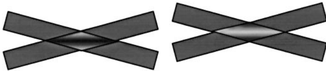
Figure 21 Effect of laser position jitter (or monitor installation jitter) on the interference pattern. The pattern does not move in space; however, the fringe that has the maximum intensity may change.
