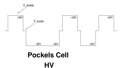
+HV: Right-handed circularly polarized light  $\rightarrow$  +Helicity electron
