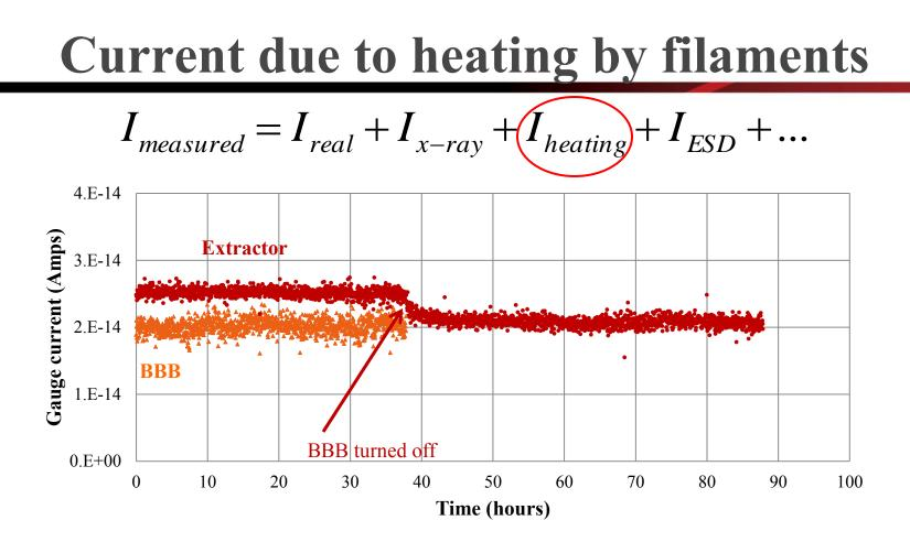
Use one gauge to measure the additional current generated by other hot filament
