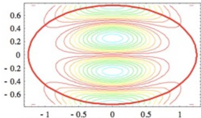
Figure 5. Electric field lines for the sTE<sub>12</sub> mode.
