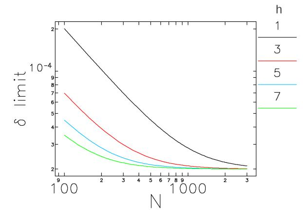
For long undulators, the maximum allowable energy shift is approximately 1/10th the rms energy spread.
