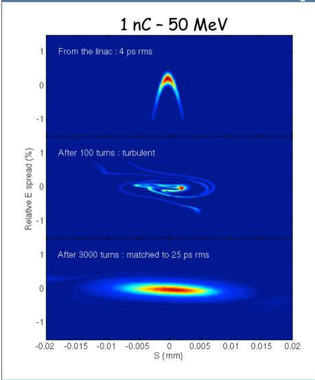
Typical longitudinal shape from the linac
