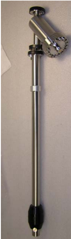
Magnetically Coupled Transporter and Valve
