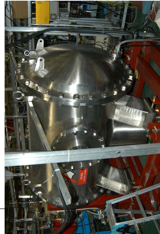
SF6 tank for JAEA thermionic cathode gun
