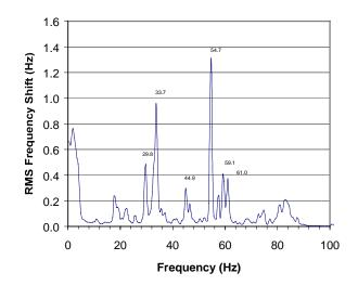
Figure 2. Actual 7-cell cavity microphonics baseline.
