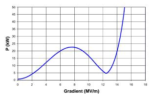
Figure 4. RF power as a function of gradient for the design parameters of the 7-cell cavity. The cavity frequency has been tuned so the cavity will be on resonance at operating field.
