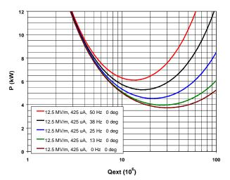
Figure 1. Forward RF power as a function of  $Q_{ext}$  at the design operating parameters of the 7-cell cavity for several amount of detuning.
