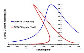
Figure 3. Resonance curves for a typical 5-cell cavity operating in CEBAF at 7.5 MV/m and  $Q_{ext}$  of 5 x 10<sup>6</sup> and for the 7-cell upgrade cavity at design gradient of 12.5 MV/m and  $Q_{ext}$  of 2.2 x 10<sup>7</sup>.
