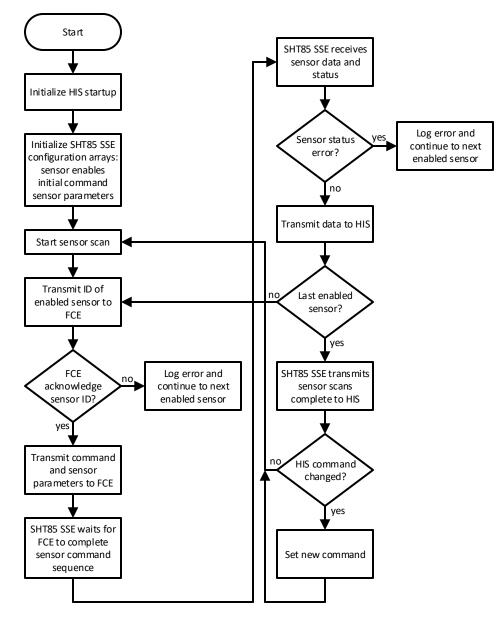
HIS = hardware interlock system SSE = system scan engine FCE = FPGA command engine
