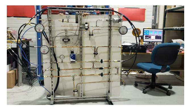
The RTPC gas system has completed JLAB pressure system requirements and is currently under testing in the JLAB EEL rm 125. The gas system will be moved to Hall B in Jan 2020.
