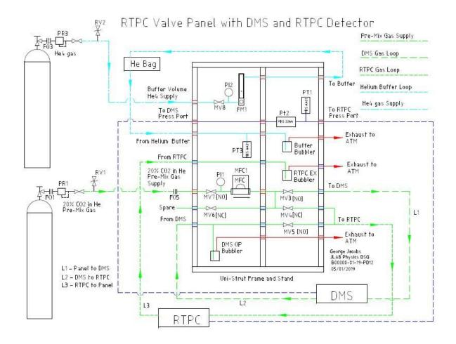
The DMS location must be outside of any magnetic field for proper operation. The DMS can be isolated and bypassed using the manual valves, MV3, MV4, and MV5.
