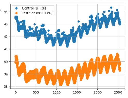
FIG. 2. Plot of control (Honeywell HIH-4030/31 series) and test (Ohmic Instruments SC-600) relative humidity sensors.
