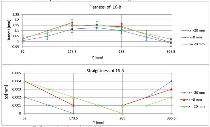
The flatness and straightness of module 16-B are in spec.
