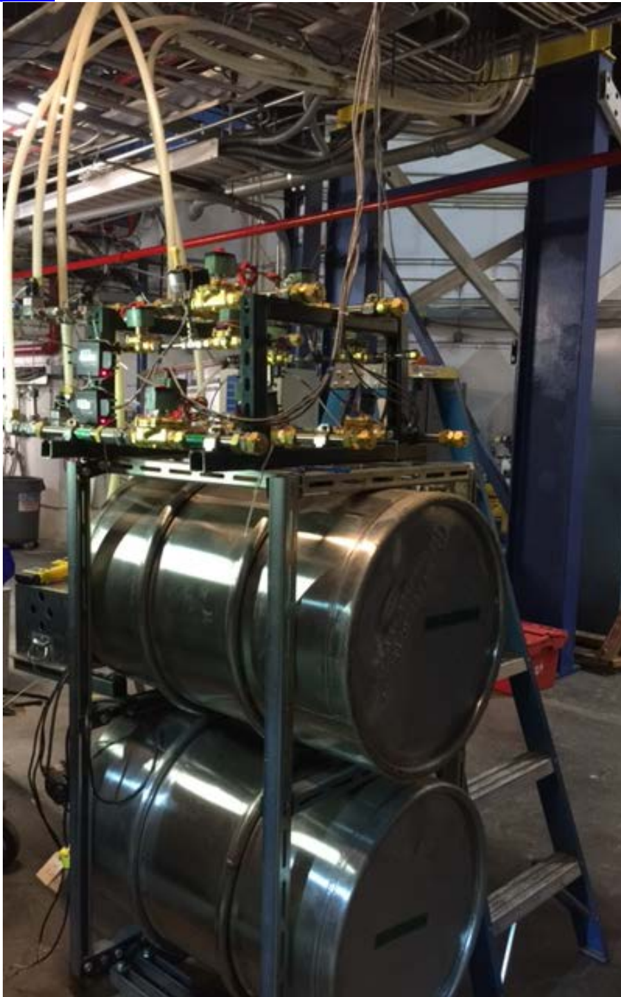
PID loop test: hardware setup
