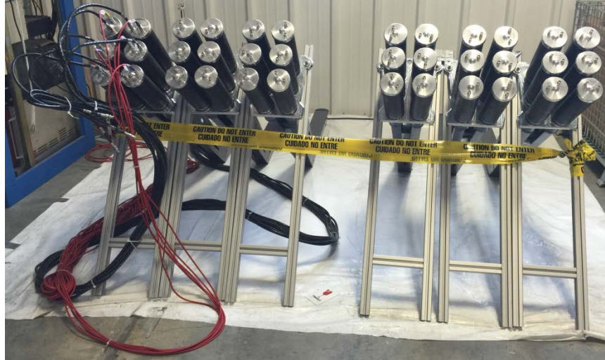
Six sets of scintillator paddles and PMTs of the CND set up in the ESB. The left-most unit was being tested and was taking cosmic data.
