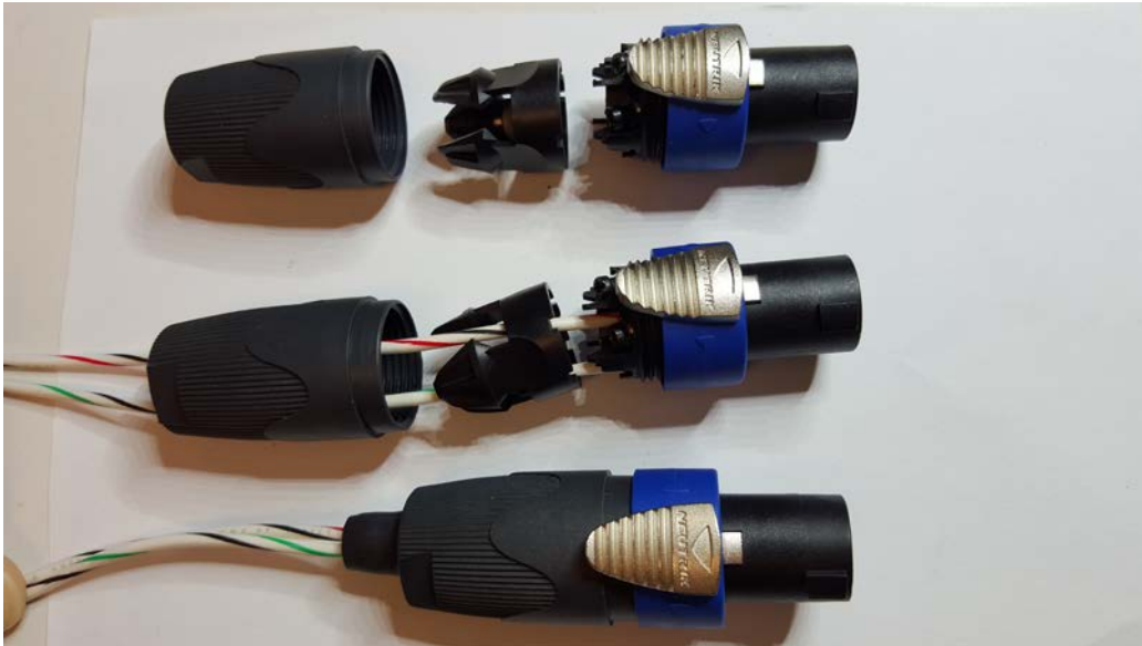
Photo of fabrication steps of compensation cable.
