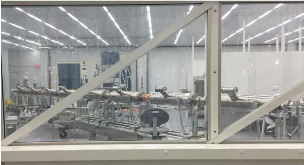
An SRF cavity string being assembled inside helium jackets. Assembly is done inside a Class 100 clean room.
