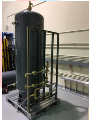
Air tank and valve panel for RICH detector
