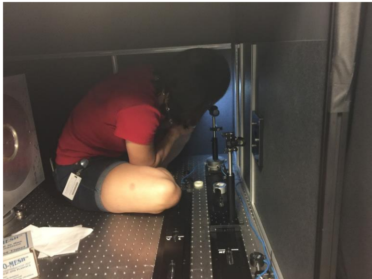
Mindy Leffel aligning optics and photodiode of test station used to measure UV transmittance.
