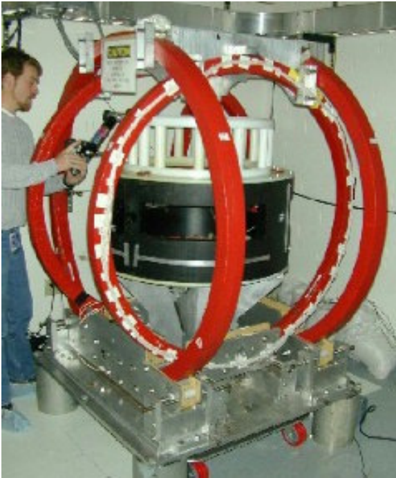
Fig.1 FaroArm Fiducialization of Hall A polarized target.
