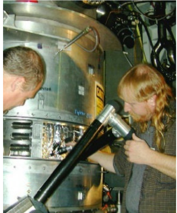
Fig. 2 Alignment of Cryo target using FaroArm
