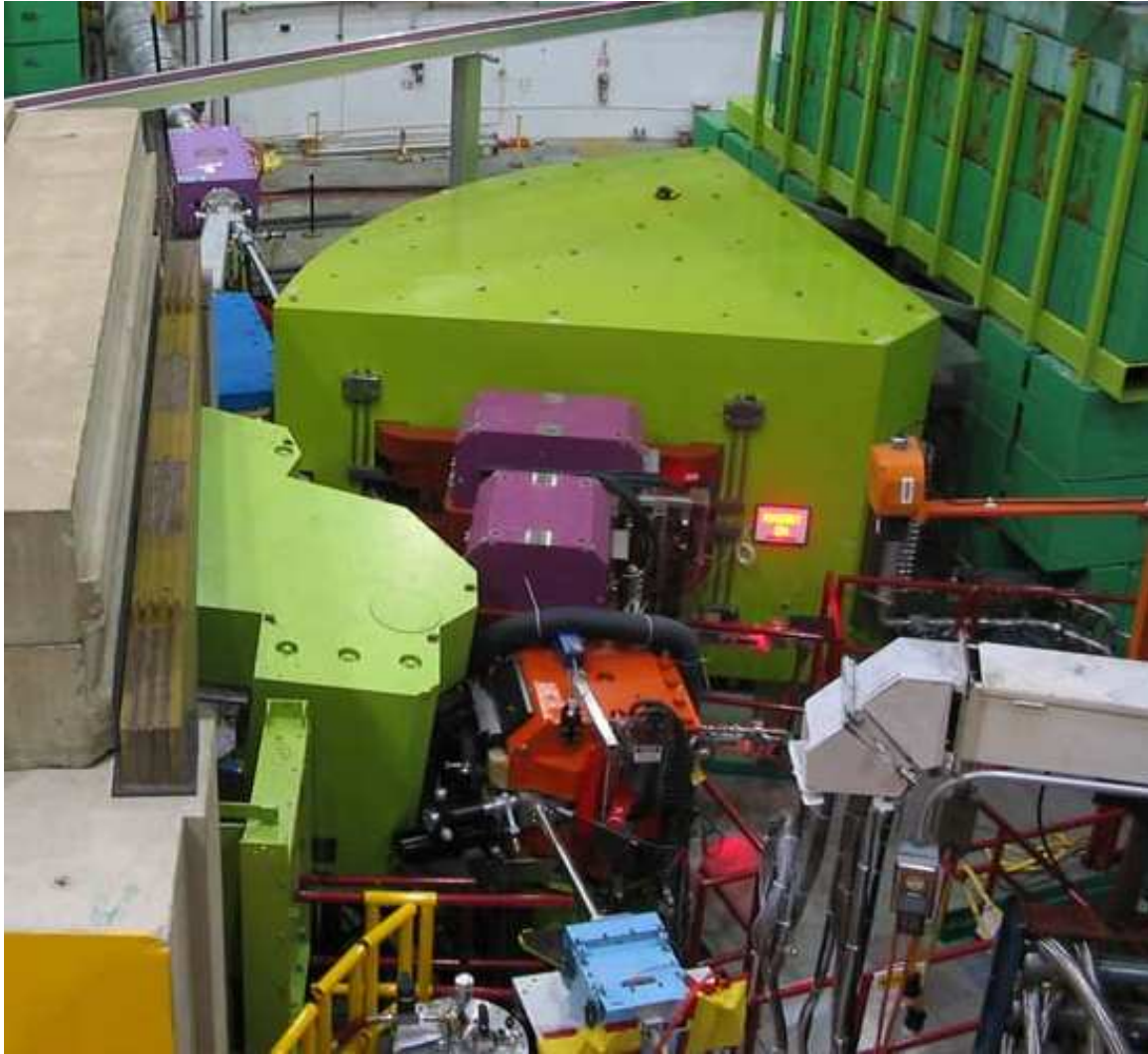
Figure 18: The HKS-ENGE setup installed in Hall C.
