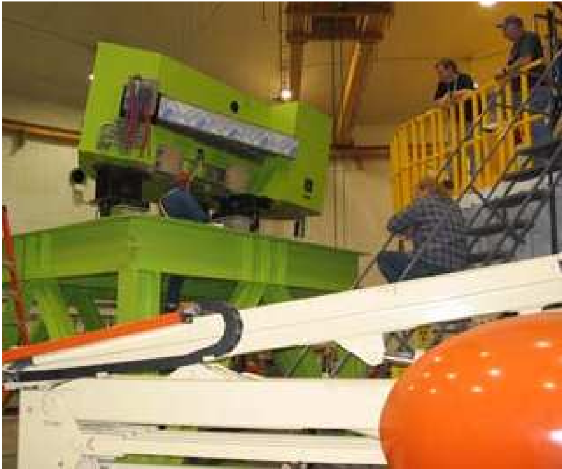
Figure 19: The ENGE spectrometer installed with a vertical tilt angle of 8 degrees in Hall C.
