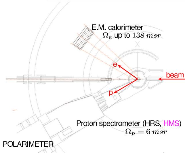
Figure 9: One High Resolution Spectrometer and one calorimeter set-up of GEP(2) in Hall A; similar set-up for the GEP(3) in Hall C.
