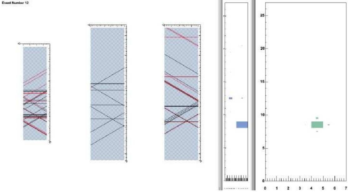
Figure 23: One event of the GEN experiment, with the BigBite arm detectors: three drift chambers and two sections of the calorimeter. The faces of the detectors are rotated to show the wires fired and the hits.
