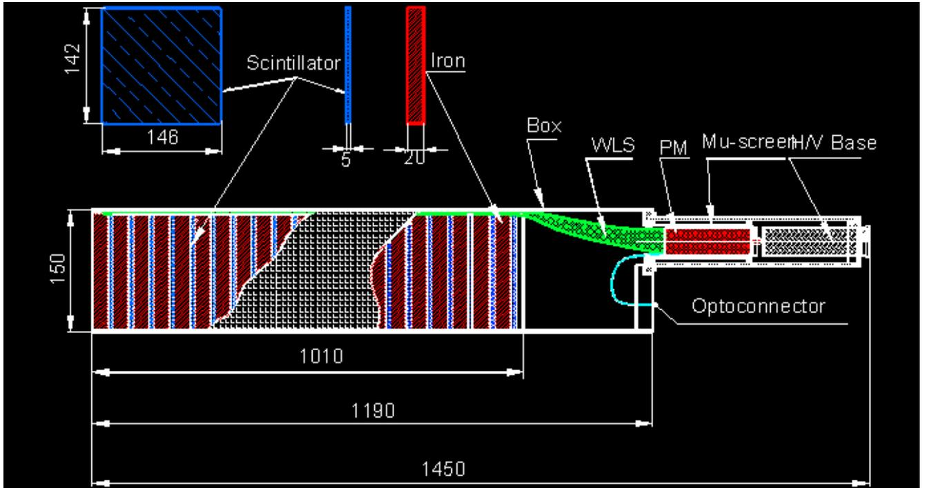
Figure 16: One module of the hadron calorimeter [84]. All dimensions are in *mm*.
