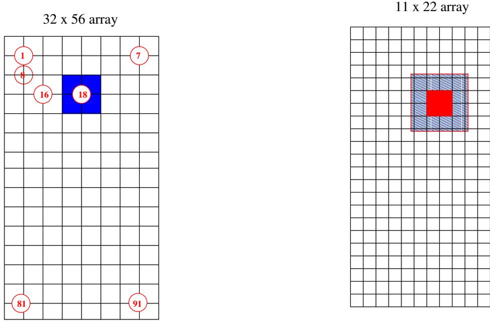
Figure 21: Trigger logic for the electron arm. The matrix of the lead-glass blocks has 32 vertical columns and 56 horizontal layers. Sums of the analog signals from each group of 4x4 blocks are sent to discriminators (for simplicity of the drawing only few sums are shown).
