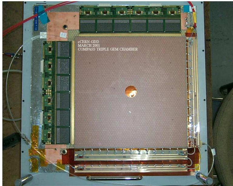
Figure 15: Triple GEM detector [83] operated in the COMPASS experiment at  $2.5 \text{ MHz/cm}^2$  rates. The hole inside is for the beam and will not be required for our application.
