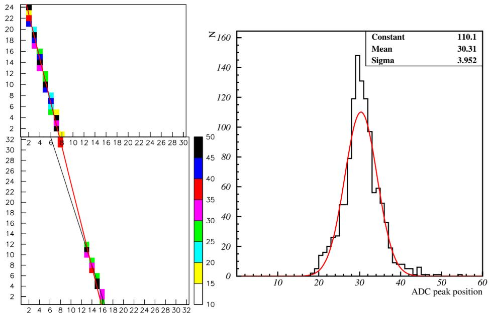
Figure 18: Left: one muon track through Protvino (bottom) and RCS (top) parts; colors represent ADC channel values, missing part of the track is in the region without HV, supposed to be supplied only in the hall. Right: ADC peak positions (in channels) after rough calibration with cosmic.
