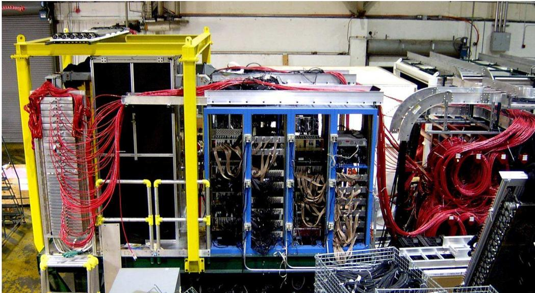
Figure 17: BigCal in Testlab, January 2007. 1744 lead-glass blocks, photo-tubes, and bases within the black box (left side with yellow frame), front-end electronics (blue racks), connected with HV (red) and signal cables (black) to the electronics platform (at the far right end).
