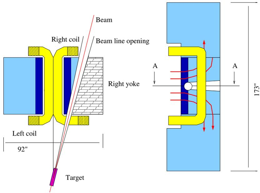
Figure 14: A sectional top view (left) and a front view (right) of the magnet. The right coil is modified to allow for the beam line passage. The beam line has a conical pipe ( $\pm 40$  mrad). The field lines (red curves in the right picture) show why the opening has just a little effect on the magnet properties.
