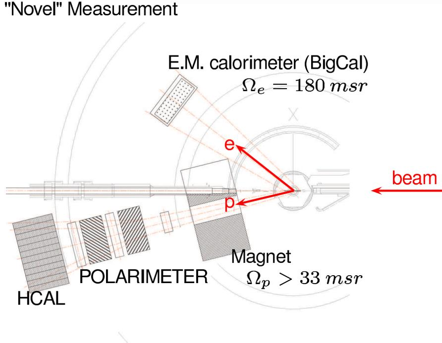
Figure 12: The proposed large acceptance setup. Proton arm: 48D48 magnet, double polarimeter with three blocks of fast tracking chambers, and a hadron calorimeter. Electron arm: 1744 channel electromagnetic calorimeter.
