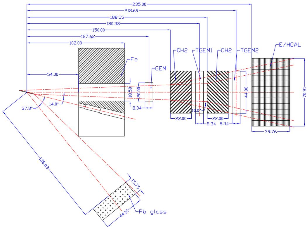
Figure 13: Detailed geometry of the proposed set-up in the reaction plane for the high  $Q^2$  measurement. All dimensions are in inches.
