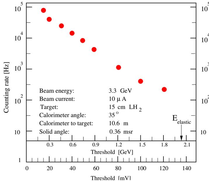
Figure 19: Typical dependence of the counting rate in the electromagnetic calorimeter vs the threshold level.
