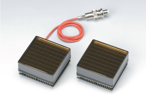
FIG. 12. The H8500 multianode photomultiplier manufactured by Hamamatsu.
