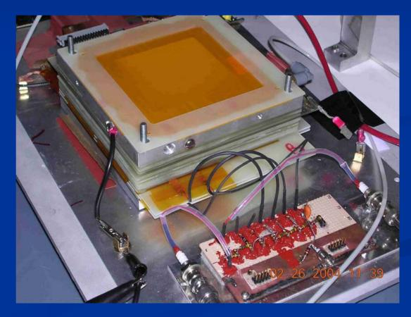
The planar prototype TPC with two new GEM foils of gain >100 at JLab
