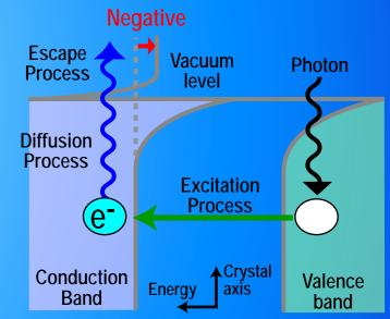
For the realization of small emittance, exciting photon energy should be tuned to band gap energy.
