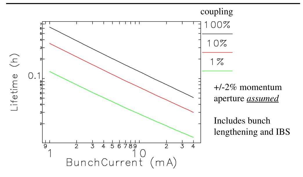
Using haissinski and ibsEmittance (L. Emery) and beamLifetimeCalc (M. Borland)
