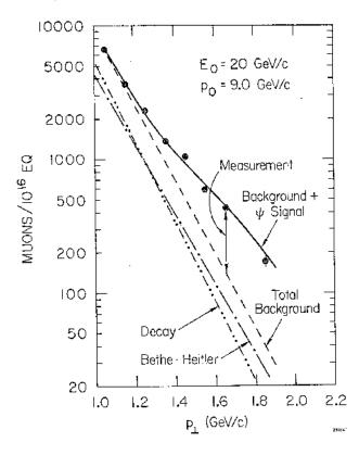
20 GeV e<sup>-</sup> on Be and Ta targets 20 GeV spectrometer,  $\mu^-$ ,  $\mu$ -filter High statistics on a high background The background was calculated: - decays
